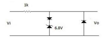
7. In the circuit shown below, assume that the voltage drop across a forward biased diode is 0.7V. The thermal voltage  $V_T = KT/q = 25$  mV. The small signal input  $V_i = V_p$  coswt where  $V_p = 100$  mV
