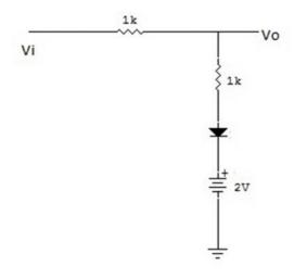
10. In the circuit shown below has to function as a clamping circuit, then what is the condition that should be satisfied for the sinusoidal signal of period T?
