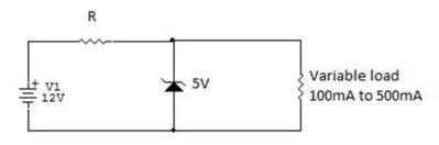
5. The zener diode in the regulator circuit shown in the figure has a zener voltage of 5.8V and a zener knee current of 0.5mA.The maximum load current drawn from this circuit ensuring proper functioning over the input voltage range between 20 and 30V is \_\_\_\_\_
